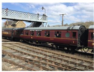
Stanier Bogie Corridor Composite (CK) Period 3 Porthole, BR Built (Diagram D2159)
