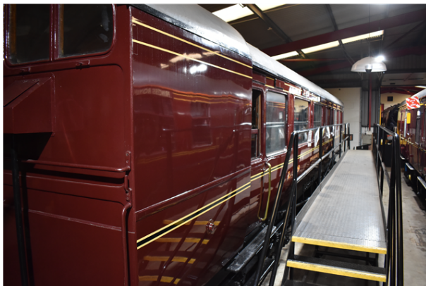
LYR 293 50' elliptical roof Dynamometer Car
