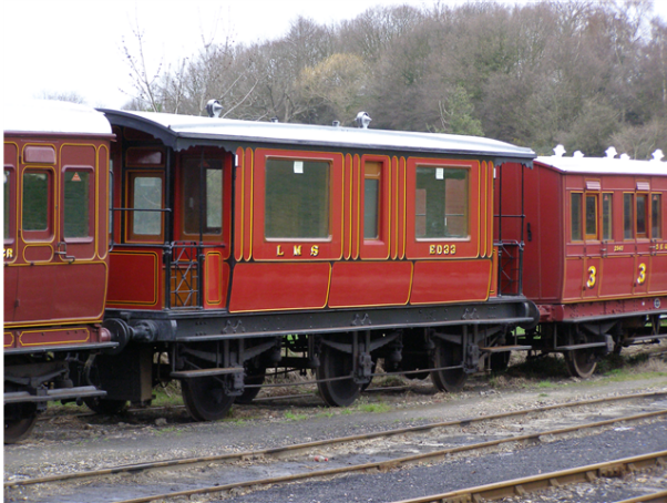
LNWR six-wheel inspection saloon
