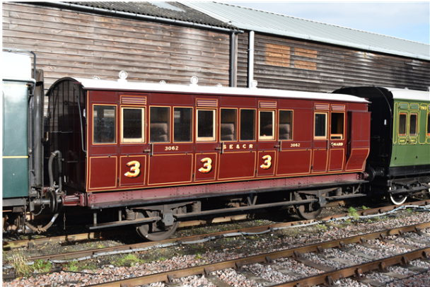
LCDR Brake Second. Body only, now running on donor underframe.
