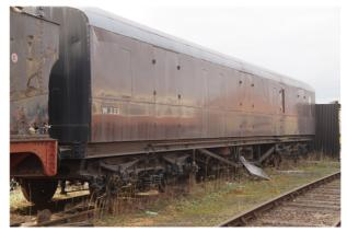
Hawksworth Bogie Gangwayed Full Brake (BG) BR Built Standard Stock (Diagram K46) Number range: W325W - W334W (10). Built Swindon Jun 1951 - Jul 1951 to Lot 1752.
