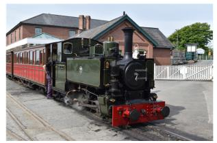
Built in 1991 using parts of 3ft gauge Andrew Barclay 0-4-0 WT for Irish turf board.
