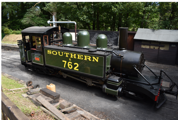
Replica new-build of line's original Baldwin locomotive.
