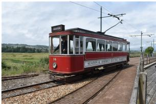
Heritage tram bodies, rebuilt with narrower body, and/or single deck to suit smaller gauge/profile.
