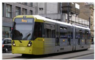
3001-3060 are fitted with ATS and VRS and can be used anywhere on the Metrolink network. These units are split between Queens Road and Trafford depots.<br/>
