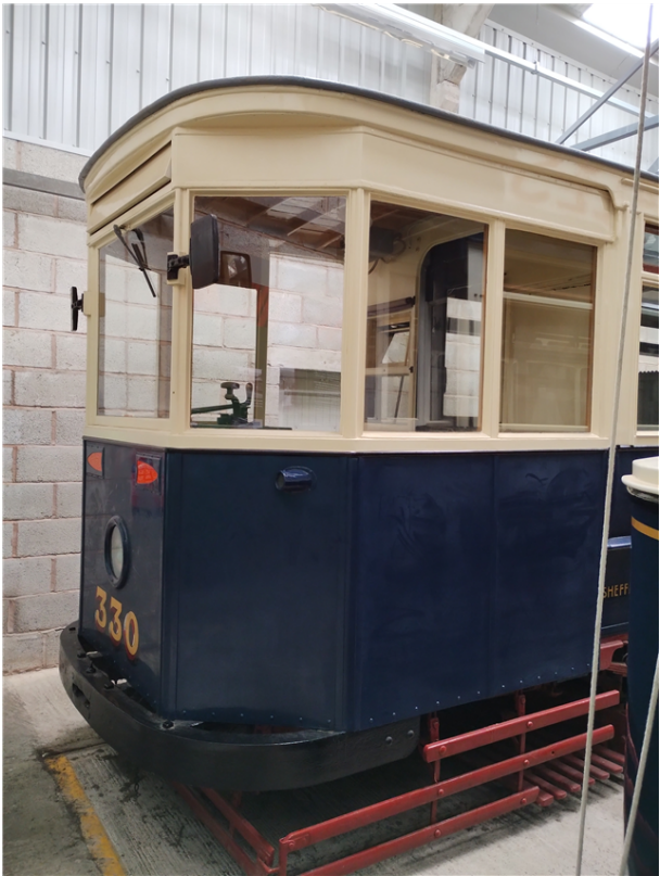
Former Bradford Corporation tram, converted as works water car / carborundum car.
