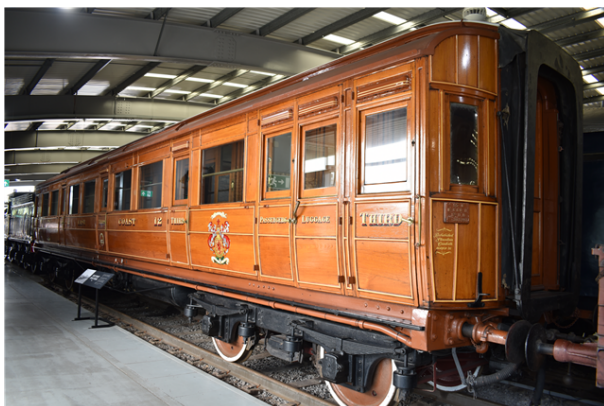
Teak construction East Coast Joint Stock Third Corridor
