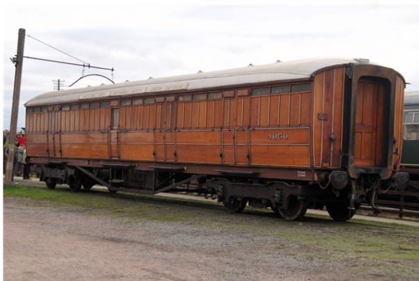
Gresley Bogie Gangway Full Brake (BGP) Pigeon Van (Diagram 315)
