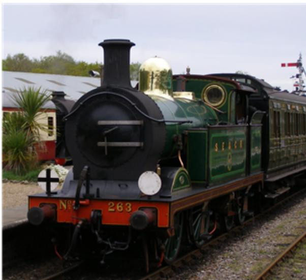
The SECR H Class is a class of 0-4-4T steam locomotive originally designed for suburban passenger work, designed by Harry Wainwright in 1904. Most of the sixty-six members of the class were later equipped for push-pull working for use on rural branch lines.
