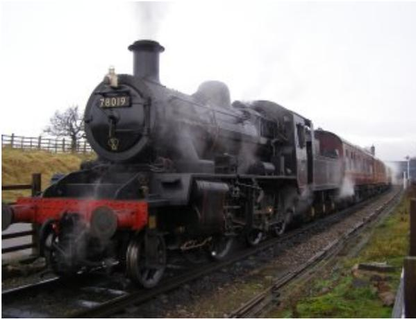
The BR Standard Class 2 2-6-0 is a class of steam locomotive, one of the British Railways Standard classes of the 1950s. They were physically the smallest of the Standard classes; 65 were built.
