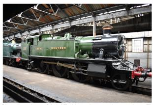
The GWR 6100 Class is a class of 2-6-2T side tank steam locomotives. The class was designed by Charles Collett and introduced in 1931 and were a straightforward development of the earlier 5101 class (and for that matter the 1905 3100/5100 class). The main difference from their predecessors was an increased boiler pressure of 225 psi with a consequent increase in tractive effort.
