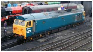
The British Rail Class 50 is a class of diesel locomotives designed to haul express passenger trains at 100 mph (160 km/h). Built by English Electric at the Vulcan Foundry in Newton-le-Willows between 1967 and 1968, the Class 50s were initially on a 10-year lease from English Electric Leasing, and were employed hauling express passenger trains on the, then non-electrified, section of the West Coast Main Line between Crewe and Scotland.
