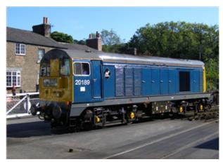
The British Rail Class 20, otherwise known as an English Electric Type 1, is a class of diesel-electric locomotive. In total, 228 locomotives in the class were built by English Electric between 1957 and 1968, the large number being in part because of the failure of other early designs in the same power range to provide reliable locomotives.
