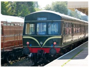
The British Rail Classes 101 and 102 diesel mechanical multiple units were built by Metro-Cammell at Washwood Heath in Birmingham, England from 1956 to 1959, following construction of a series of prototype units. These classes proved to be some of the most successful and longest-lived of BR's First Generation DMUs.
