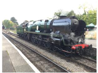
Due to problems with some of the new features, such as the Bulleid chain-driven valve gear, sixty locomotives were rebuilt by British Railways during the late 1950s. The results were similar to the rebuilt Merchant Navy class.
