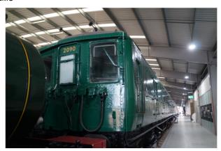
The Southern Railway (SR) gave the designation 2-BIL to the DC third rail electric multiple units built during the 1930s to work long-distance semi-fast services on the newly electrified lines from London to Eastbourne, Portsmouth and Reading. This type of unit survived long enough in British Rail ownership to be allocated TOPS Class 401.
