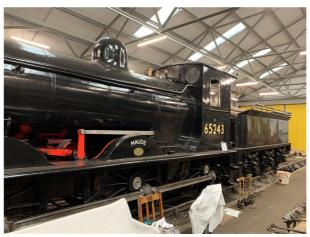
The NBR C Class (LNER Class J36) is a class of 0-6-0 steam locomotives designed by Matthew Holmes for freight work on the North British Railway (NBR). They were introduced in 1888 with inside cylinders and Stephenson valve gear.
