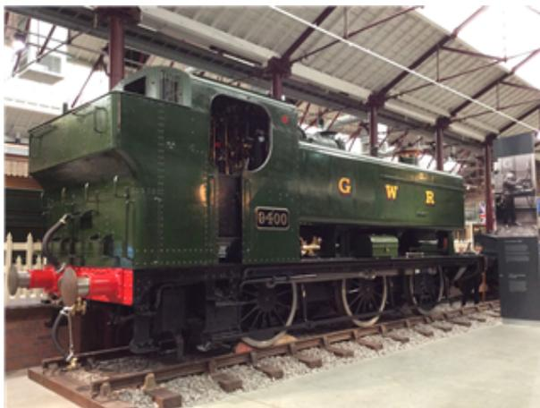
The Great Western Railway (GWR) 9400 Class is a class of 0-6-0 pannier tank steam locomotive, used for shunting and banking duties.
