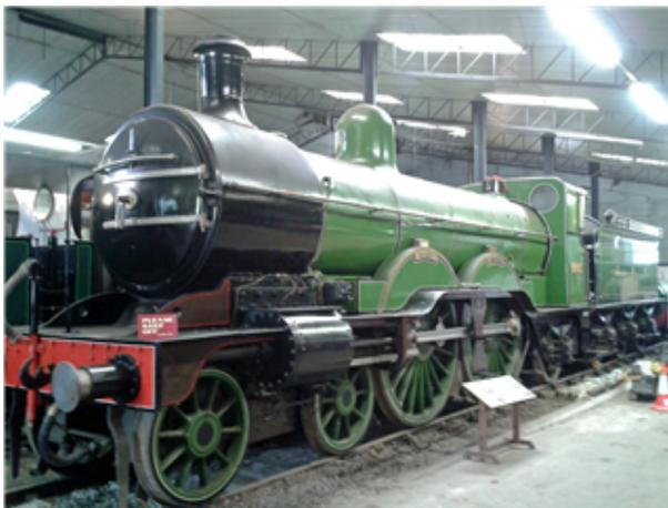
The GNR Small Boiler Class C1 is a class of steam locomotive, the first 4-4-2 or Atlantic type in Great Britain. They were designed by Henry Ivatt in 1897. In total 22 were built between 1898 and 1903 at Doncaster Works. They could reach speeds of up to 90 mph. They were also known as Klondykes.
