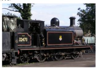
The LB&SCR E4 class is a class of 0-6-2T side tank steam locomotive designed by Robert Billinton. They were introduced in 1897 and were essentially a larger version of the E3 Class. They were powerful for their size and were stalwarts of local passenger, freight and branch work for more than fifty years.
