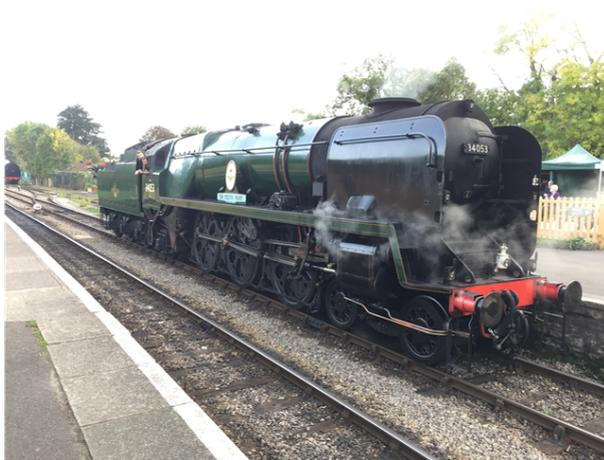
Due to problems with some of the new features, such as the Bulleid chain-driven valve gear, sixty locomotives were rebuilt by British Railways during the late 1950s. The results were similar to the rebuilt Merchant Navy class.
