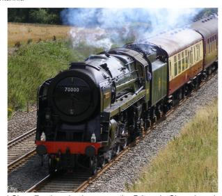
The BR Standard Class 7, otherwise known as the Britannia Class, is a class of 4-6-2 Pacific steam locomotive designed under Robert Riddles for use by British Railways for mixed-traffic duties. 55 were constructed between 1951 and 1954. The design employed results from the 1948 locomotive exchanges undertaken in advance of further locomotive
