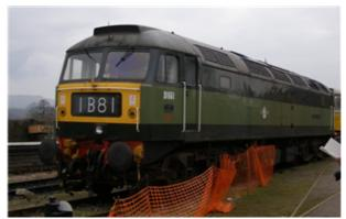
The British Rail Class 47 or Brush Type 4 is a class of diesel-electric locomotive that was developed in the 1960s by Brush Traction. A total of 512 Class 47s were built at Brush's Falcon Works in Loughborough and at British Railways' Crewe Works between 1962 and 1968, which made them the most numerous class of British mainline diesel locomotive.
