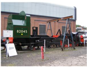
The BR Standard Class 3 2-6-2T was a class of steam locomotive designed by Robert Riddles for British Railways. It was essentially a hybrid design, the chassis being closely based on and sharing a number of parts with the LMS Ivatt Class 4, and having a boiler derived from a GWR No.2 boiler as fitted to the GWR Large Prairie 2-6-2T and 5600 Class 0-6-2T tank engines.
