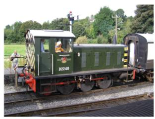
The British Rail Class 04 is a 0-6-0 diesel-mechanical shunting locomotive class, built between 1952 and 1962 and was the basis for the later Class 03 built in the British Railways workshops.
