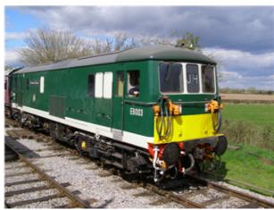
The British Rail Class 73 is a British electro-diesel locomotive. The type is unusual in that it can operate from the Southern Region's 650/750 V DC third-rail or an on-board diesel engine to allow it to operate on non-electrified routes. This makes it very versatile, although the diesel engine produces less power than is available from the third-rail supply, so the locomotives are rarely operated outside of the former Southern Region of British Rail.
