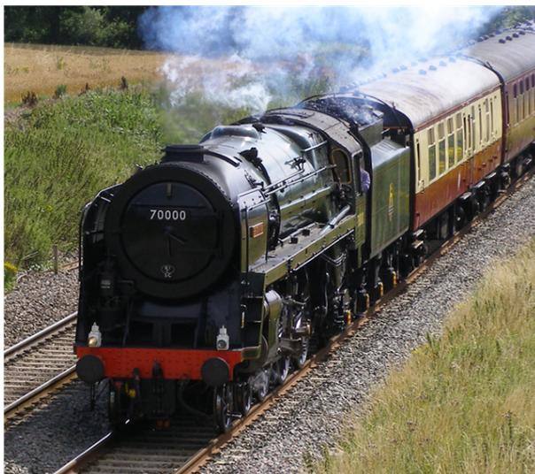
The BR Standard Class 7, otherwise known as the Britannia Class, is a class of 4-6-2 Pacific steam locomotive designed under Robert Riddles for use by British Railways for mixed-traffic duties. 55 were constructed between 1951 and 1954. The design employed results from the 1948 locomotive exchanges undertaken in advance of further locomotive classes being constructed. Three batches were constructed at Crewe Works, before the publication of the 1955 Modernisation Plan.
