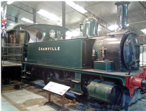
The LSWR B4 class is a class of 0-4-0 tank engines originally designed for station piloting and dock shunting. They were later used extensively in Southampton Docks for nearly half a century.
