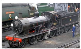
The LSWR T9 class was a class of 66 4-4-0 steam locomotive designed for express passenger work by Dugald Drummond and introduced to services on the LSWR in 1899. One example has been preserved after British Railways ownership. They were given the nickname of "Greyhounds" due to their speed, up to 85 miles per hour, and reliability.
