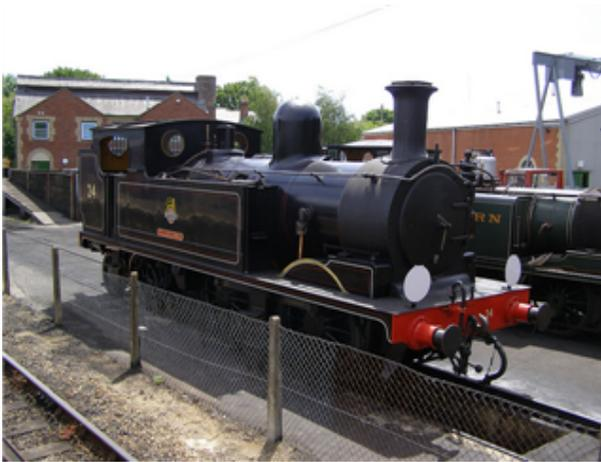
The LSWR O2 class is a class of 0-4-4T steam locomotive designed for the LSWR by William Adams. Sixty were constructed during the late nineteenth century. They were also the last steam engines to work on the Isle of Wight, with the final two being withdrawn in 1967.
