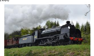
The LSWR S15 class is a British 2-cylinder 4-6-0 freight steam locomotive designed by Robert W. Urie, based on his H15 class and N15 class locomotives. The class had a complex build history, spanning several years of construction from 1920 to 1936.
