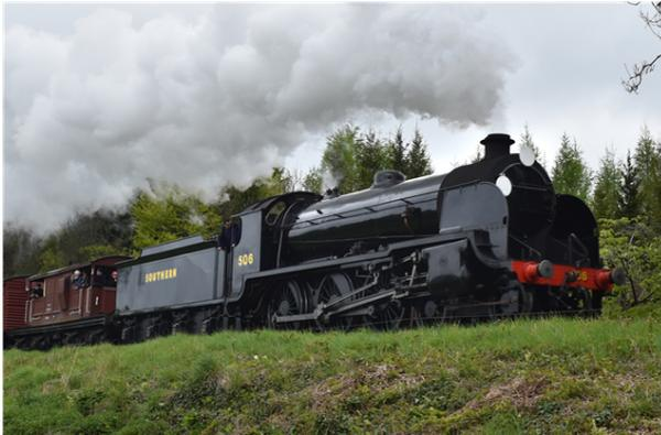
The LSWR S15 class is a British 2-cylinder 4-6-0 freight steam locomotive designed by Robert W. Urie, based on his H15 class and N15 class locomotives. The class had a complex build history, spanning several years of construction from 1920 to 1936.
