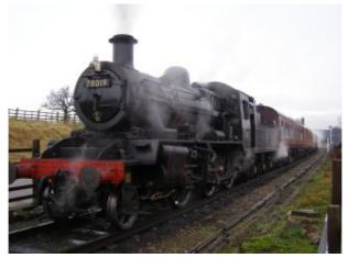
The BR Standard Class 2 2-6-0 is a class of steam locomotive, one of the British Railways Standard classes of the 1950s. They were physically the smallest of the Standard classes; 65 were built.
