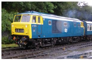
The British Rail Class 35 is a class of mixed-traffic B-B diesel locomotive with hydraulic transmission. Because of their Mekydro-design hydraulic transmission units, the locomotives became known as the Hymeks. They were numbered D7000-D7100.
