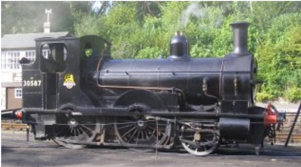
The LSWR 0298 Class or Beattie Well Tank is a class of British steam locomotive. They are 2-4-0WTs, originally built between 1863 and 1875 for use on passenger services in the suburbs of London, but later used on rural services in Southwest England. Out of a total production of 85, two locomotives have been preserved in an operational condition.
