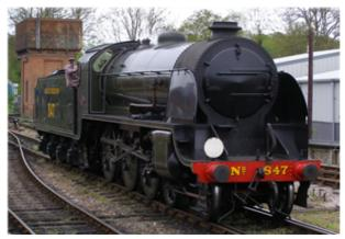
The LSWR S15 class is a British 2-cylinder 4-6-0 freight steam locomotive designed by Robert W. Urie, based on his H15 class and N15 class locomotives. The class had a complex build history, spanning several years of construction from 1920 to 1936.
