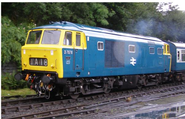
The British Rail Class 35 is a class of mixed-traffic B-B diesel locomotive with hydraulic transmission. Because of their Mekyll-design hydraulic transmission units, the locomotives became known as the Hymeks. They were numbered D7000-D7100.
