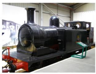
The LB&SCR E1 Class were 0-6-0T steam locomotives designed by William Stroudley in 1874 for short-distance goods and piloting duties. They were originally classified E, and generally known as "E-tanks"; They were reclassified E1 in the time of D. E. Marsh.
