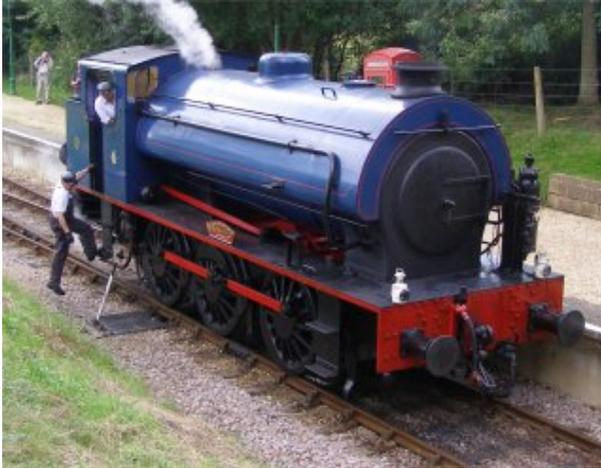
The Hunslet Austerity 0-6-0ST is a class of steam locomotive designed by Hunslet Engine Company for shunting. The class became the standard British shunting locomotive during the Second World War, and production continued until 1964 at various locomotive manufacturers.
