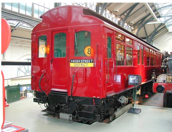
Q23-stock was the name given to modernised ex-G- stock cars. The G-stock was introduced to the District line in 1923. These cars were fitted with hand-operated doors and were nicknamed 'horse boxes' because of their narrow cabs. In 1938 this stock was modernised so that it could run with the new Q38 stock. The modernised cars had automatic doors and electro-pneumatic brakes.
