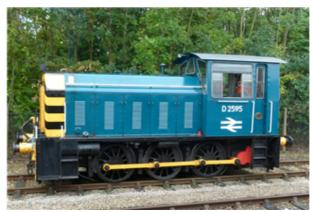
The British Rail Class 05 is a class of 0-6-0 diesel-mechanical shunters built by Hunslet Engine Company from 1955 to 1961. They were used on the Eastern and Scottish Regions of British Railways. The first two batches were delivered as 11136-11143 (later renumbered D2550-D2557) and 11161-11176 (later renumbered D2558-D2573). Subsequent locomotives were delivered, new, as D2574-D2618.
