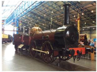
The Furness Railway No.3, nicknamed "Old Coppernob", is a preserved English steam locomotive. It acquired its nickname because of the copper cladding to its dome-shaped "haystack" firebox.
