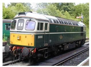
The British Rail Class 33, also known as the BRCW Type 3 or Crompton, is a class of Bo-Bo diesel-electric locomotives, ordered in 1957 and built for the Southern Region of British Railways between 1960 and 1962.
