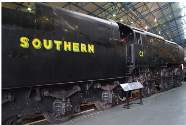
The SR Q1 class is a type of austerity steam locomotive constructed during the Second World War. The class was designed by Oliver Bulleid for use on the intensive freight turns experienced during wartime on the Southern Railway network. A total of 40 locomotives were built. Bulleid incorporated many innovations and weight-saving concepts to produce a highly functional design.
