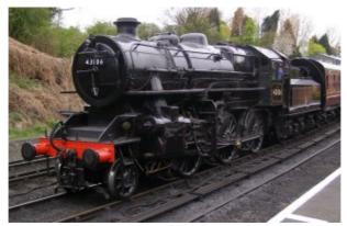
The LMS Ivatt Class 4 2-6-0 is a class of steam locomotive primarily designed for medium freight work but also widely used on secondary passenger services. The LMS ordered 162 of this type between 1947 and 1952, but only three were built by the LMS before nationalisation in 1948. Designed by George Ivatt, they were classified 4F by the LMS and 4MT by BR.
