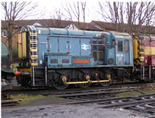
The British Rail Class 10 diesel locomotive was a variant of the standard Class 08 diesel-electric shunter with a Lister Blackstone diesel engine and General Electric Company plc (GEC) traction motors. The locomotives were built at the BR Works in Darlington and Doncaster over the period 1955–1962, and were withdrawn between February 1967 and June 1972.
