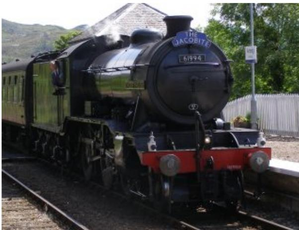
The LNER Class K4 is a class of 2-6-0 steam locomotives designed by Nigel Gresley for the steep grades of the West Highland Line.
