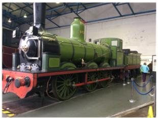
The NER 1001 Class was a class of long-boiler 0-6-0 steam locomotive designed in Britain by William Bouch.
