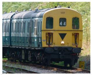
The British Rail Class 207 (3D) diesel-electric multiple units were built by BR at Eastleigh in 1962. The fleet had a lifespan of 42 years. The Southern Region class 201 to 207 DEMUs are nicknamed 'Thumpers' due to the noise their engine units make.
