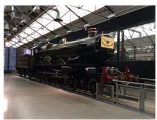
The 4073 or Castle Class are 4-6-0 steam locomotives of the Great Western Railway, built between 1923 and 1950. They were designed by the railway's Chief Mechanical Engineer, Charles Collett, for working the company's express passenger trains. They could reach speeds of up to 100 mph.
