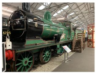
The LNER D40 class is a type of 4-4-0 steam locomotive inherited from the GNSR. It consisted of GNSR class V (introduced in 1899 by William Pickersgill) and GNSR class F (introduced in 1920 by T. E. Heywood). The two classes were similar, but the class F was superheated.
