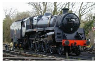
The British Railways Standard Class 5MT 4-6-0 is one of the 12 standard classes of steam locomotive built by British Railways in the 1950s. It was essentially a development of the LMS Stanier Class 5 4-6-0 ("Black Five") which had been the most successful mixed-traffic type in Great Britain.
