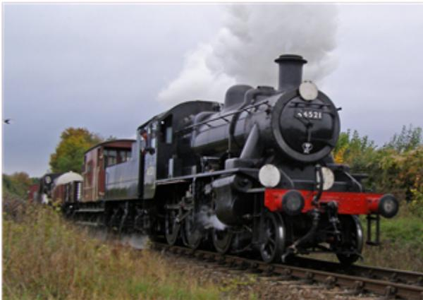
The London, Midland and Scottish Railway (LMS) Ivatt Class 2 2-6-0 is a class of steam locomotive designed for light mixed traffic. Elderly 0-6-0s formed the backbone of the low-powered locomotives within the LMS fleet. William Stanier had concentrated on introducing larger engines and it was left to George Ivatt to introduce a new class of low-powered locomotive. He designed a tender version of the Ivatt Class 2 2-6-2T
