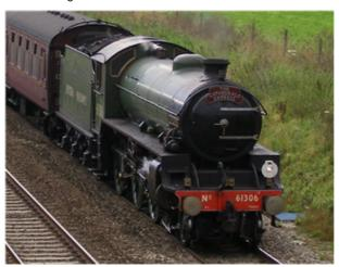
The LNER Thompson Class B1 is a class of steam locomotive designed by Edward Thompson for medium mixed traffic work. It was the LNER's equivalent to the highly successful GWR Hall Class and the LMS Stanier Black Five, two-cylinder mixed traffic 4-6-0s. However, it had the additional requirement of having to be cheap because, due to wartime and post-war economies, the LNER, never the richest railway company, had to make savings.
