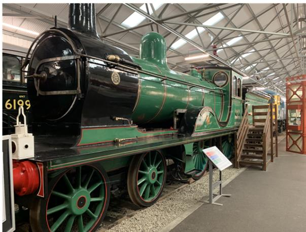
The LNER D40 class is a type of 4-4-0 steam locomotive inherited from the GNSR. It consisted of GNSR class V (introduced in 1899 by William Pickersgill) and GNSR class F (introduced in 1920 by T. E. Heywood). The two classes were similar, but the class F was superheated.
