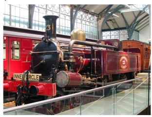
The Metropolitan Railway A Class and B Class were 4-4-0T condensing steam locomotives built for the Metropolitan Railway by Beyer Peacock, first used in 1864. A total of 40 A Class and 26 of the slightly different B Class were delivered by 1885. Used underground, the locomotives condensed their steam, and coke or smokeless coal was burnt to reduce the smoke.
