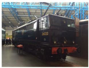
The British Rail Class 76, also known as Class EM1 (Electric Mixed-Traffic 1), is a class of 1.5 kV DC, Bo-Bo electric locomotive designed for use on the now-closed Woodhead Line in Northern England.
