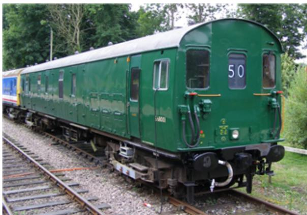
The British Rail Class 419 Motor Luggage Vans (or MLV) were battery electric multiple unit cars built from 1951-61 by BR at Eastleigh Works. Each MLV unit is essentially a motorised BG carriage, with a driver's position at each end. Each vehicle has two luggage compartments and a guard's compartment.
