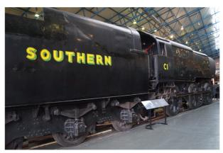
The SR Q1 class is a type of austerity steam locomotive constructed during the Second World War. The class was designed by Oliver Bulleid for use on the intensive freight turns experienced during wartime on the Southern Railway network. A total of 40 locomotives were built. Bulleid incorporated many innovations and weight-saving concepts to produce a highly functional design.
