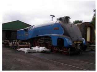
The Class A4 is a class of streamlined 4-6-2 steam locomotive designed by Nigel Gresley for the LNER in 1935. Their streamlined design gave them high-speed capability as well as making them instantly recognisable, and one of the class 4468 Mallard, holds the world record as the fastest steam locomotive.
