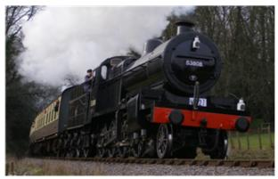
The Somerset and Dorset Joint Railway (S&DJR) 7F 2-8-0 is a class of steam locomotive designed for hauling heavy coal and goods trains. Eleven were built in two batches in 1914 and 1925 and were used until withdrawal between 1959 and 1964.
