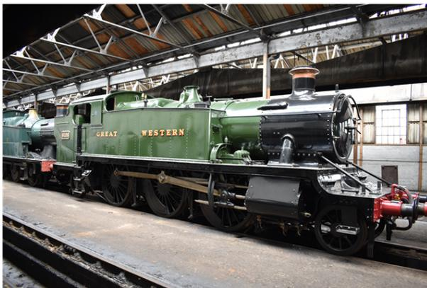
The GWR 6100 Class is a class of 2-6-2T side tank steam locomotives. The class was designed by Charles Collett and introduced in 1931 and were a straightforward development of the earlier 5101 class (and for that matter the 1905 3100/5100 class). The main difference from their predecessors was an increased boiler pressure of 225 psi with a consequent increase in tractive effort.
