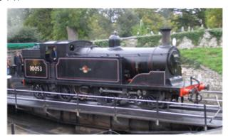
The LSWR M7 class is a class of 0-4-4T passenger tank locomotive built between 1897 and 1911. The class was designed by Dugald Drummond for use on the intensive London network of the LSWR and performed well in such tasks.
