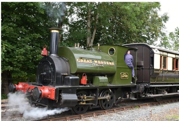
GWR No. 1340 is an 0-4-0ST steam locomotive, built in 1897 (Works No. 1386) by the Avonside Engine Company of Bristol, England. Its first owners were Messrs Dunn & Shute of
