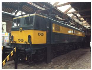
The British Rail Class 77, also known as Class EM2, is a class of 1.5 kV DC, Co-Co electric locomotive. They were built by Metropolitan-Vickers in 1953–1954 for use over the Woodhead Line between Manchester and Sheffield.
