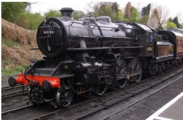
The LMS Ivatt Class 4 2-6-0 is a class of steam locomotive primarily designed for medium freight work but also widely used on secondary passenger services. The LMS ordered 162 of this type between 1947 and 1952, but only three were built by the LMS before nationalisation in 1948. Designed by George Ivatt, they were classified 4F by the LMS and 4MT by BR.
