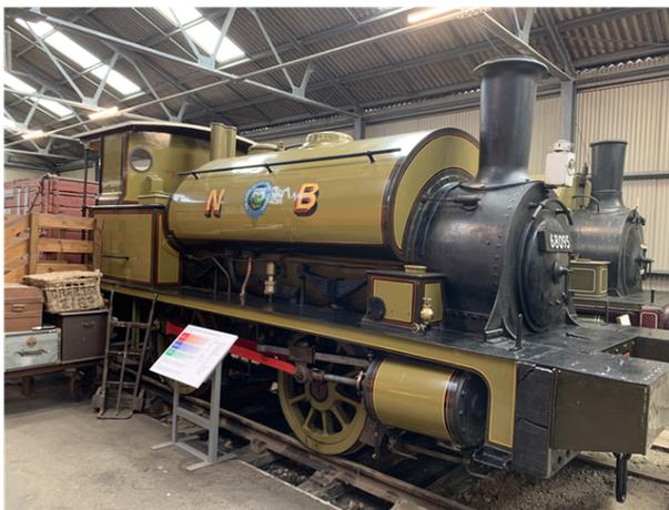
The NBR G Class (LNER Class Y9) is a class of 0-4-0ST steam locomotive designed for shunting. Some locomotives were equipped with small wooden tenders to carry extra coal. They were introduced in 1882 and thirty-eight entered service on the NBR between 1882 and 1899. Like most 0-4-0 tanks of the period, it has outside cylinders and inside slide valves driven by Stephenson valve gear.
