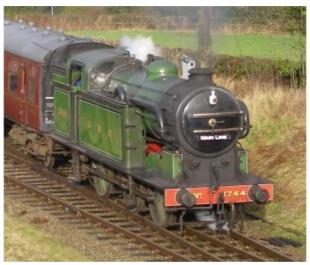
The GNR Class N2 is an 0-6-2T side tank steam locomotive designed by Nigel Gresley and introduced in 1920. Further batches were built by the LNER from 1925. They had superheaters and piston valves driven by Stephenson valve gear. Some locomotives were fitted with condensing apparatus for working on the Metropolitan Railway Widened Lines between King's Cross and Moorgate.
