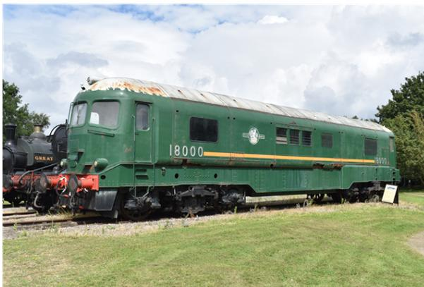
British Rail 18000 was a prototype mainline gas turbine-electric locomotive built for British Railways in 1949 by Brown, Boveri & Cie. An earlier gas-turbine locomotive, 18100, had been ordered from Metropolitan-Vickers by the Great Western Railway but construction was delayed due to World War II; a second, 18000, was thus ordered from Switzerland in 1946. It spent its working life on the Western Region of British Railways, operating express passenger services from Paddington station, London.
