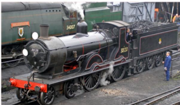
The LSWR T9 class was a class of 66 4-4-0 steam locomotive designed for express passenger work by Dugald Drummond and introduced to services on the LSWR in 1899. One example has been preserved after British Railways ownership. They were given the nickname of "Greyhounds" due to their speed, up to 85 miles per hour, and reliability.
