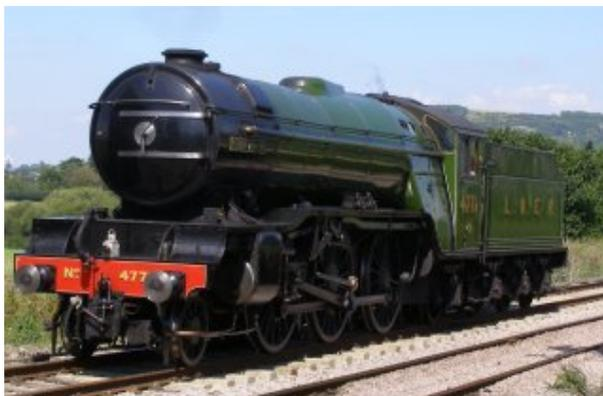
The LNER Class V2 2-6-2 steam locomotives were designed by Sir Nigel Gresley for express mixed traffic work and were built at the LNER shops at Doncaster and Darlington between 1936 and 1944. The best known is the first of the class, 4771 (later 800 and 60800) Green Arrow, which is the sole survivor of the class.
