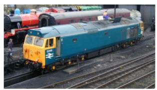
The British Rail Class 50 is a class of diesel locomotives designed to haul express passenger trains at 100 mph (160 km/h). Built by English Electric at the Vulcan Foundry in Newton-le-Willows between 1967 and 1968, the Class 50s were initially on a 10-year lease from English Electric Leasing, and were employed hauling express passenger trains on the, then non-electrified, section of the West Coast Main Line between Crewe and Scotland.
