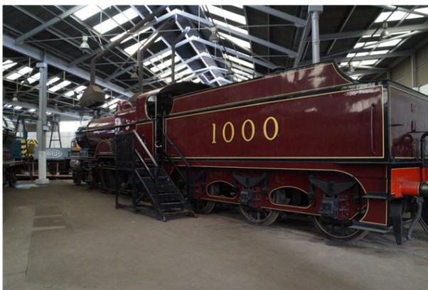
Midland Railway 1000 Class is a class of 4-4-0 steam locomotive designed for passenger work. They were known to reach speeds of up to 85 mph. They were developed from a series of five locomotives (2631-2635) introduced in 1902 by Samuel Waite Johnson, which
