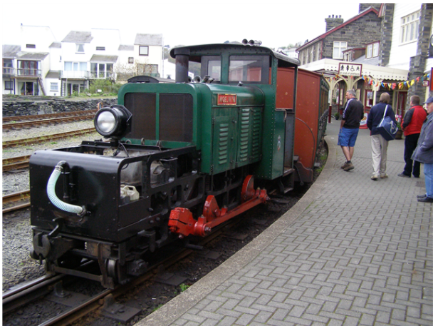
Baldwin diesel built in 1918 for WWI use as 0-4-0. Rebuilt as 2-4-0
