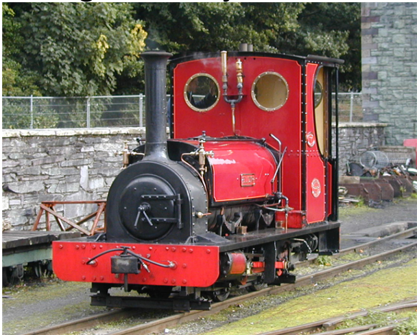
Hunslet 0-4-0 Loco's built for use in North Wales Penrhyn Quarry. This is the large variant of the Penrhyn Quarry Hunslet
