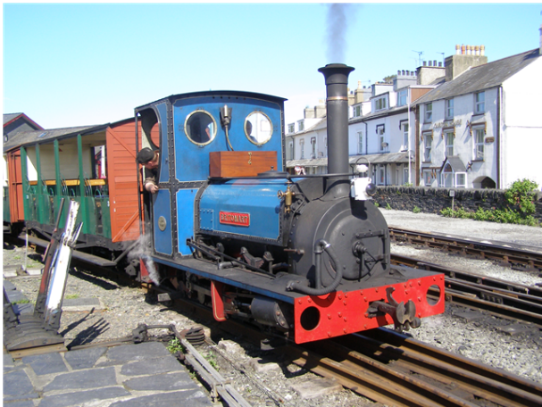
Hunslet Quarry Tanks, built for and used in various North Wales quarries.
