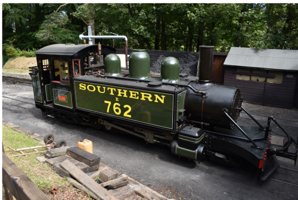
Replica new-build of line's original Baldwin locomotive.
