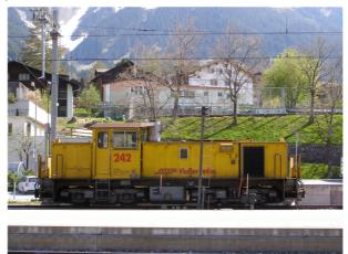
Originally used for construction of Vereina tunnel. Now used for works and construction duties.
