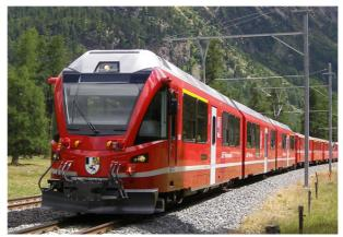
Allegra units. Dual voltage units capable of operating over the entire RhB network.
