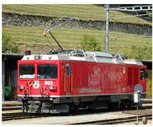
Electro-Diesel locos, these can be used on the Bernina DC electric, or on diesel. The loco's are normally found on the Bernina line.
