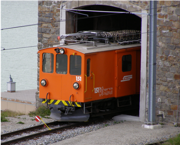
Former motor luggage van, rebuilt as shunting locomotive. Bernina line.
